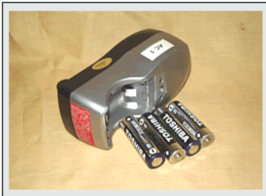
Battery charger and four rechargeable batteries
